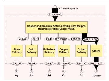
Figure 3. Schematic diagram of global potential recovery of five selected precious metals (Ag, Au, Pd, Cu, Co) from PCs/ Laptops (values are reported in Mg/a) [13]
